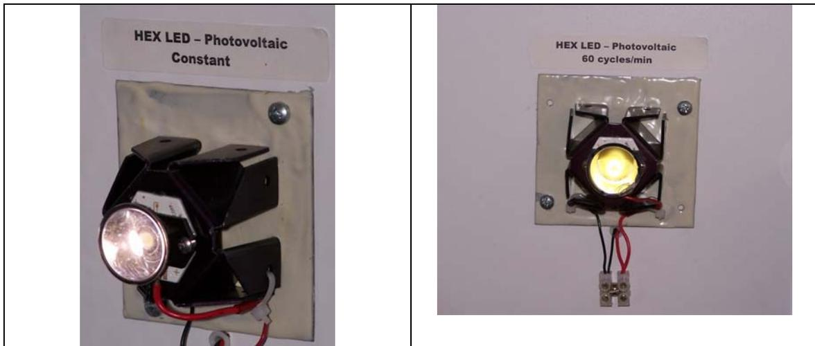
**Figure 3. PV powered Norlux white Hex under test at SWRES.**
